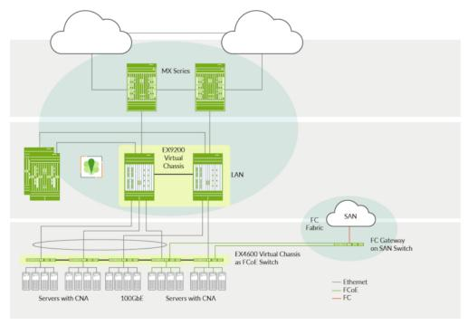
$\textit{Figure 6:} \ \textit{The EX4600 can be deployed as a data center FCoE transit switch in a top-of-rack Virtual Chassis configuration. } \\$
